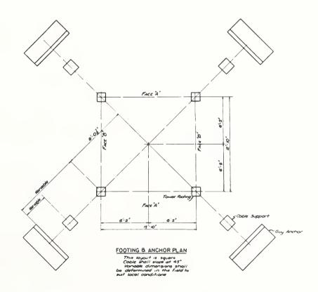
Figure 69. A typical tower footing plan. This was designed for a CT-2 timber lookout tower.
